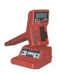
Investigators performed a detailed study of the parameters affecting a locating device's ability to function in various soil types and conditions. It was determined that soil conductivity and relative dielectric constant, both highly dependent on soil moisture contents, are the two key parameters for most pipelocation techniques.
