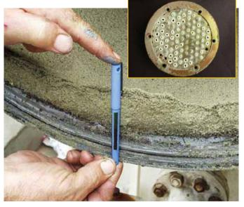
Elemental sulfur can significantly restrict or even stop the flow of gas through operations equipment.
