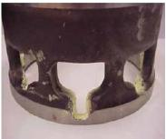
Control valve cage with elemental sulfur deposition.
