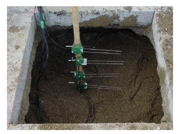
Moisture and temperature instrumentation in a bellhole.
