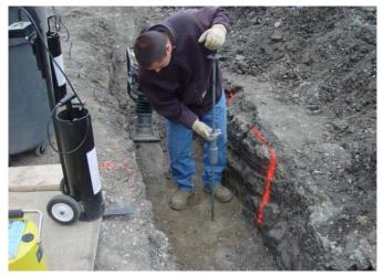
Soil-compaction measurement devices were tested at GTI's Pipe Farm and at several utility sites.
