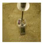
The DCP uses a five-pound drop-weight to drive a small cone into the soil, counting the number of drops required to penetrate the soil a fixed distance of 3-<sup>1</sup>/<sub>4</sub> inches. The number of drops is determined by calibrating the device to the relative soil compaction of various soil types. Researchers report that the device proved to be a practical replacement for the nuclear density gauge by providing layer-by-layer compaction verification.
