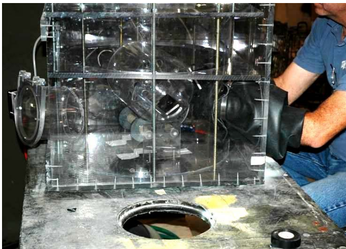
A special chamber was designed and built to conduct the measurements and tests in a flammable mixture.
