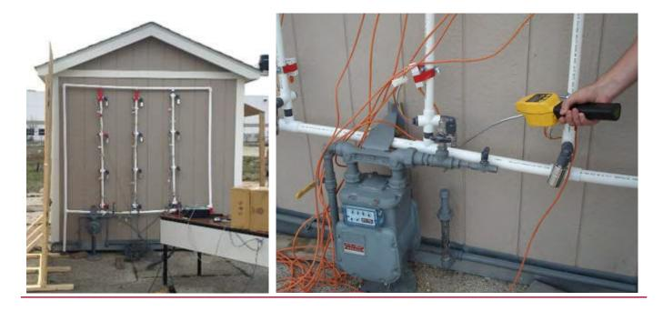
performed in an outdoor building at the Gas Technology Institute testing facility. An array of gas sensors were used to monitor gas concentrations from 0% to 100% gas at 15-inch intervals and at various locations around the leak source.
