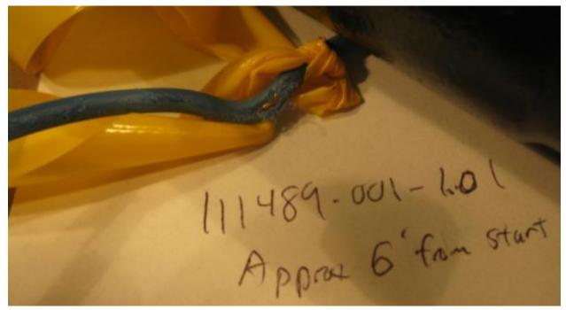
Figure 13. Break of Insulation Jacket (#1) on Field Tested Company A-12 AWG Solid Copper Wire
