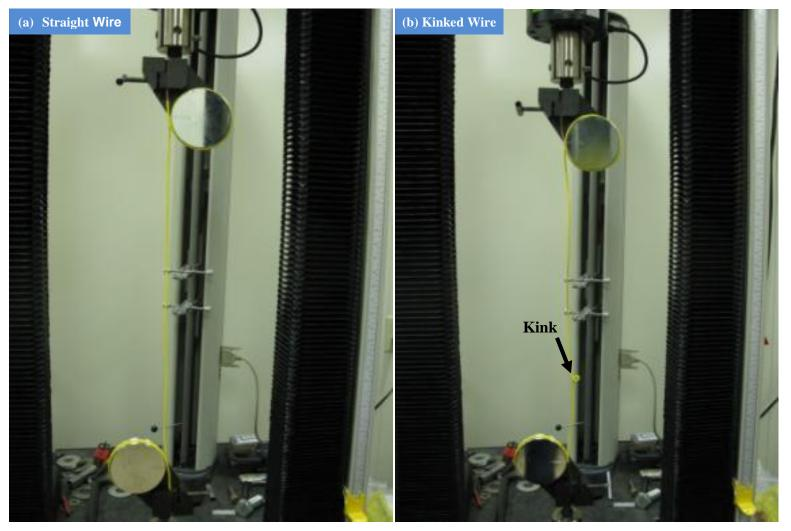
Figure 2. Wire Tensile Test Setup
