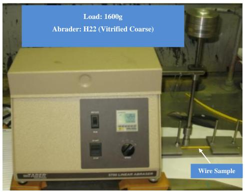
Figure 3. Taber Abrasion Test Setup
