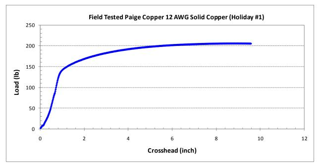
Figure 41. Tensile Plot for Field Tested Company C 12 AWG Solid Copper Wire (Holiday #1)
