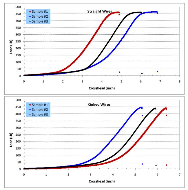
Figure 35. Tensile Plots for Straight and Company B 10 AWG Hard Drawn Copper Wire
