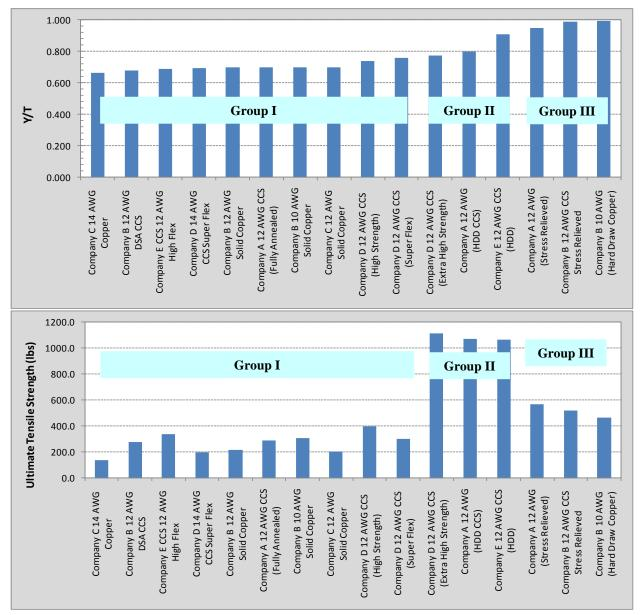
Figure 7. The Y/T vs. the Ultimate Tensile Strength of Straight Tracer Wires
