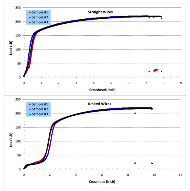
Figure 22. Tensile Plots for Straight and Kinked Company B 12 AWG Soft Drawn Copper Wire
