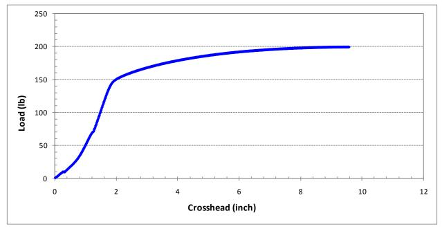
Figure 38. Tensile Plot for Field Tested Company A 12 AWG Copper Clad Steel Wire (Holiday #1)
