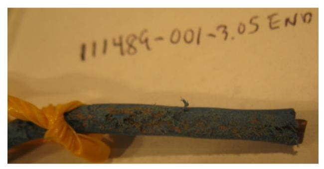
Figure 16. Break of Insulation Jacket (#4) on Field Tested Company A-12 AWG Solid Copper Wire
