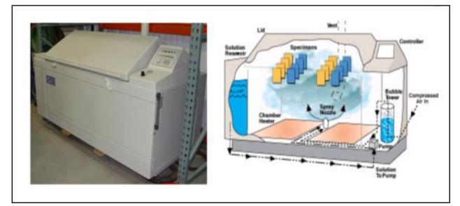
Figure 9. Cyclic Salt Fog Tester
