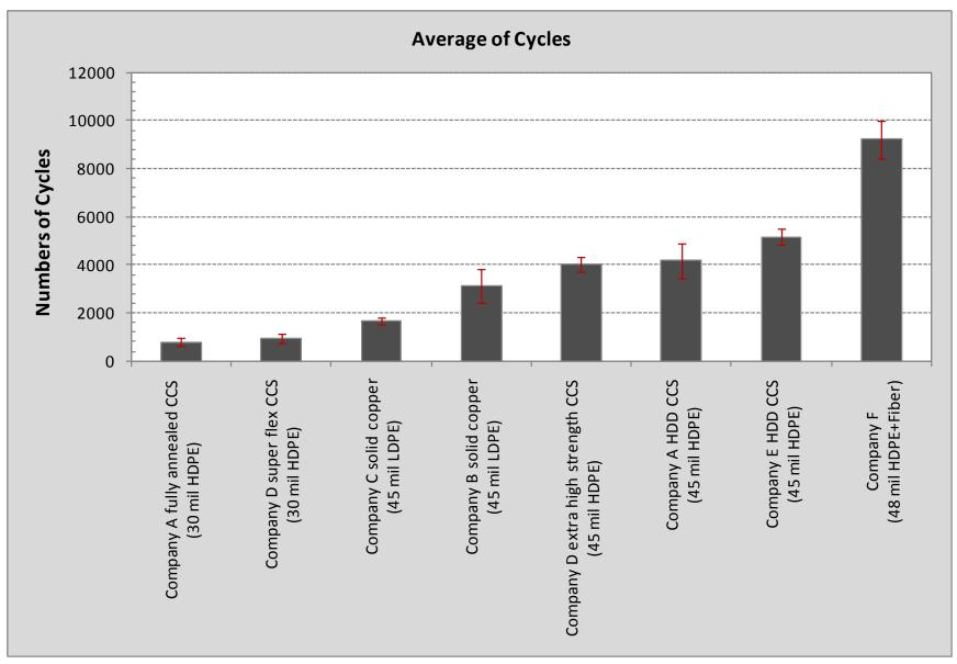
Figure 6. Scrape Test Results
