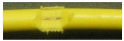
**Figure 5. Wire Sample after Scrape Test**
