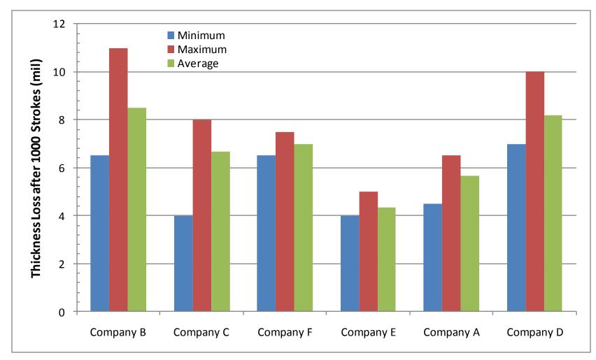
**Figure 4. Taber Abrasion Test Results**
