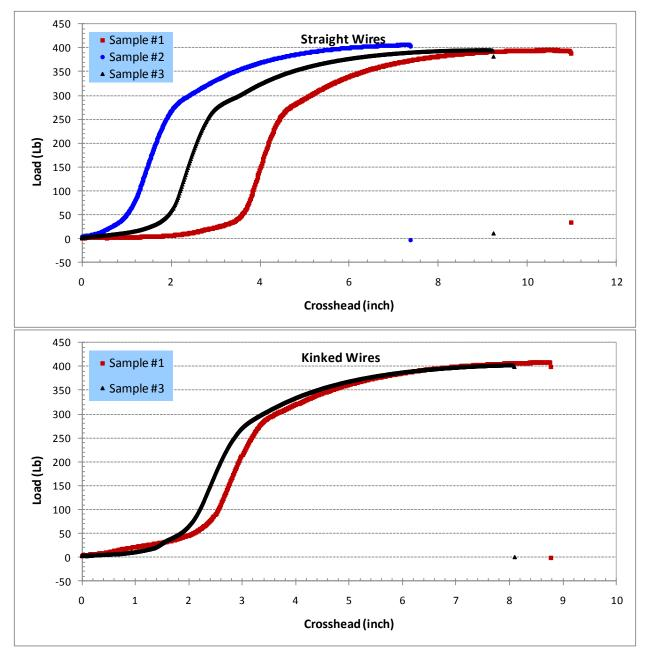
Figure 32. Tensile Plots for Straight and Kinked Company D 12 AWG High Strength Copper Clad Steel Wire
