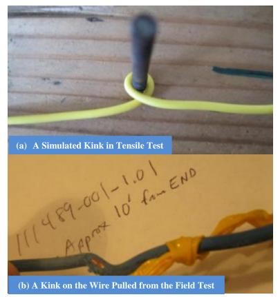
Figure 1. The Simulated Kink for Tensile Test vs. a Kink on the Field Tested Wire
