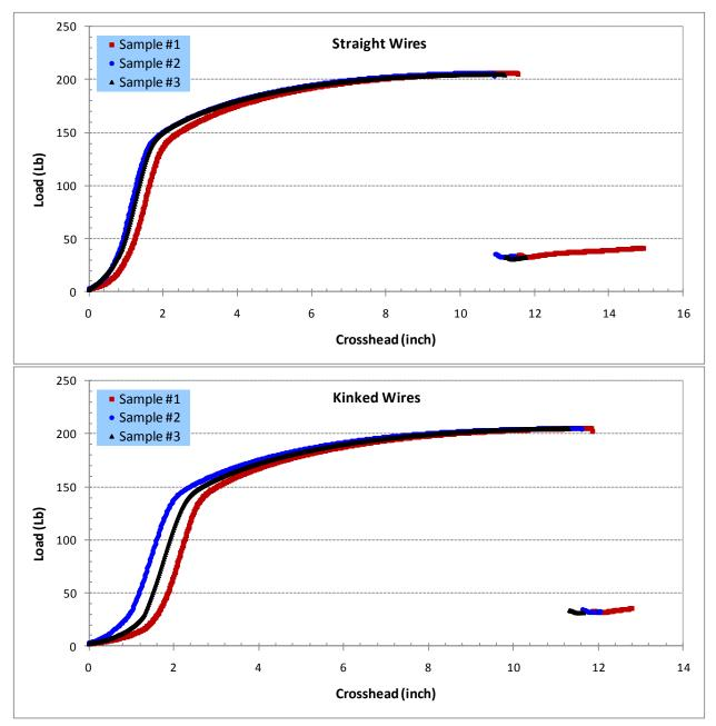
Figure 21. Tensile Plots for Straight and Kinked Company C 12 AWG Copper Wire
