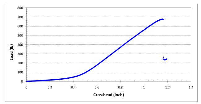
Figure 40. Tensile Plot for Field Tested Company E HDD 12 AWG Copper Clad Steel Wire
