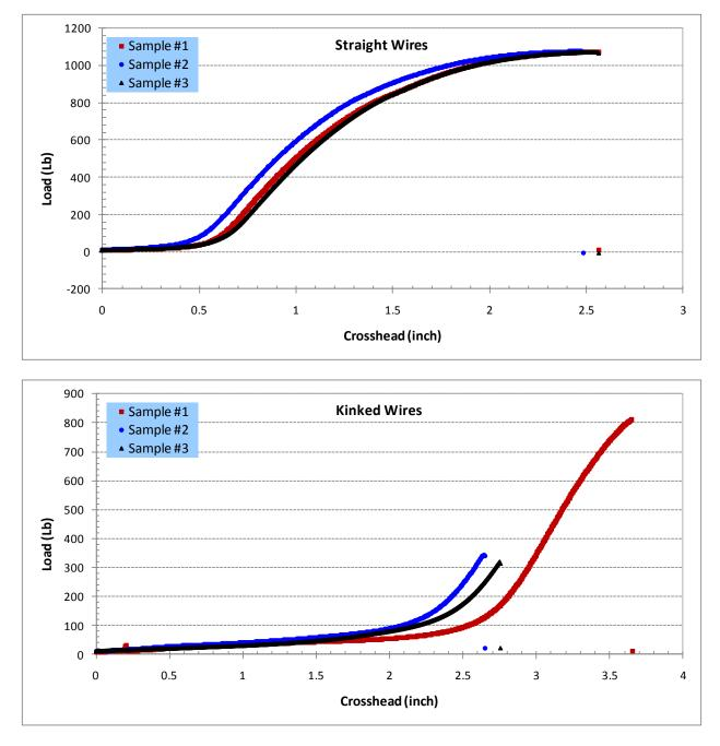
Figure 28. Tensile Plots for Straight and Kinked Company A HDD 12 AWG Copper Clad Steel Wire
