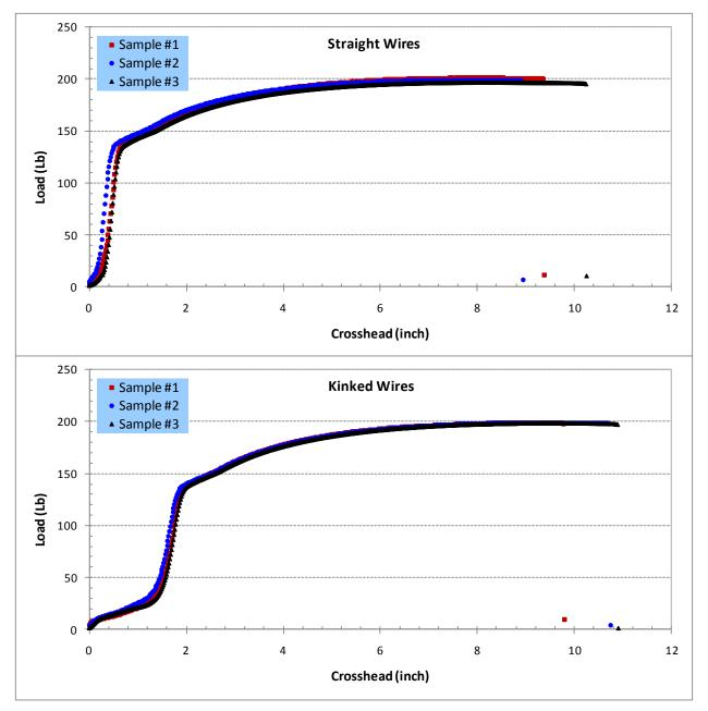
Figure 23. Tensile Plots for Straight and Kinked Company D 14 AWG Super Flex Soft Drawn Copper Clad Steel Wire
