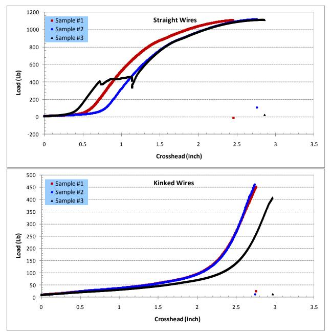
Figure 30. Tensile Plots for Straight and Kinked Company D Extra High Strength 12 AWG Copper Clad Steel Wire
