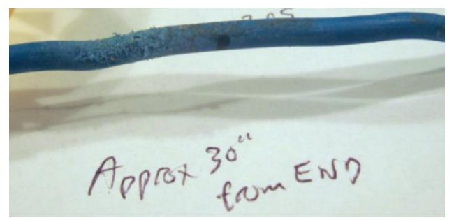
Figure 15. Break of Insulation Jacket (#3) on Field Tested Company A-12 AWG Solid Copper Wire
