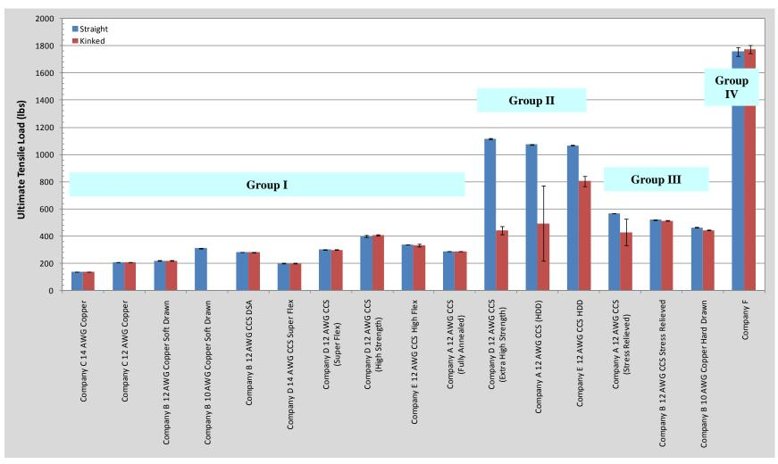
Figure 8. Ultimate Tensile Strength of the Straight and Kinked Tracer Wires
