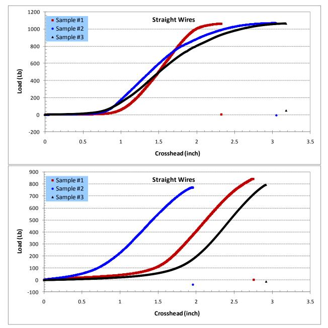
Figure 29. Tensile Plots for Straight and Kinked Company E HDD 12 AWG Copper Clad Steel Wire
