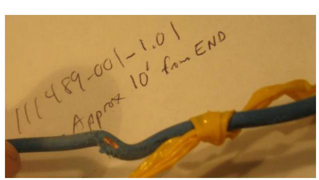
Figure 14. Break of Insulation Jacket (#2) on Field Tested Company A-12 AWG Solid Copper Wire
