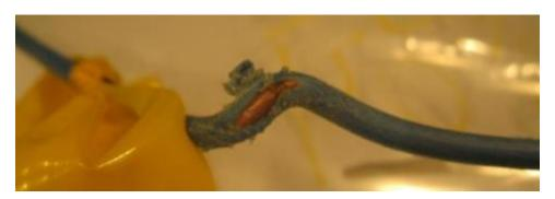
Figure 19. Break of Insulation Jacket (#3) on Field Tested Company D-12 AWG Copper Clad Steel Wire
