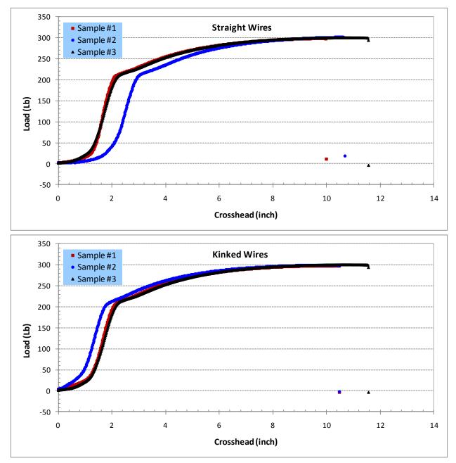
Figure 24. Tensile Plots for Straight and Kinked Company D 12 AWG Super Flex Copper Clad Steel Wire
