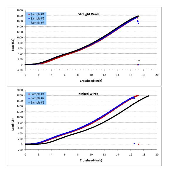
Figure 31. Tensile Plots for Company F Wire (Straight and Kinked)
