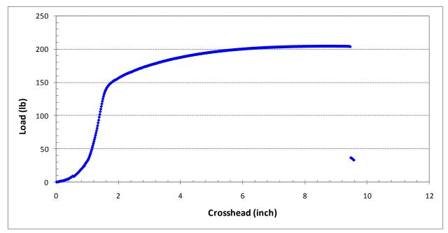
Figure 42. Tensile Plot for Field Tested Company C 12 AWG Copper Wire (Holiday #2)
