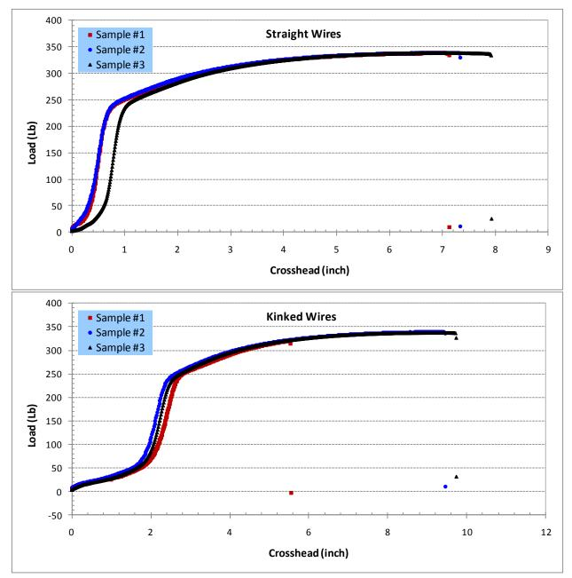
Figure 25. Tensile Plots for Straight and Kinked Company E High Flex 12 AWG Copper Clad Steel Wire
