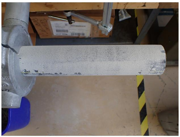
Figure 161. Pipe contaminated with bentonite powder
