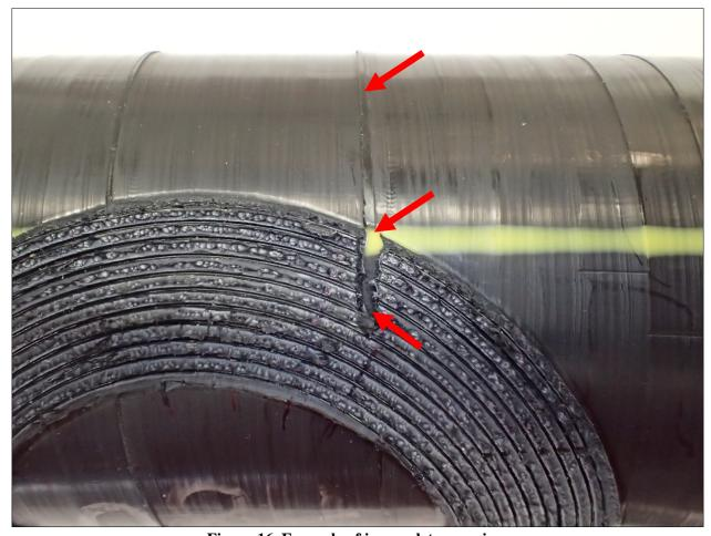
Figure 16. Example of incomplete scraping
