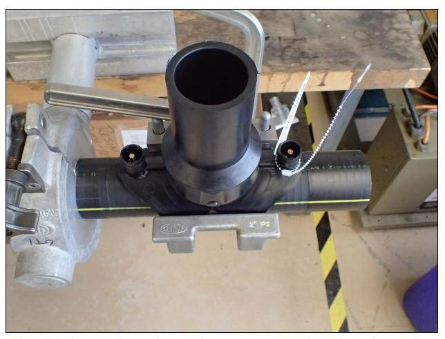
Figure 166. Pipe contaminated with bentonite powder, saddle clamping promptly after scraping
