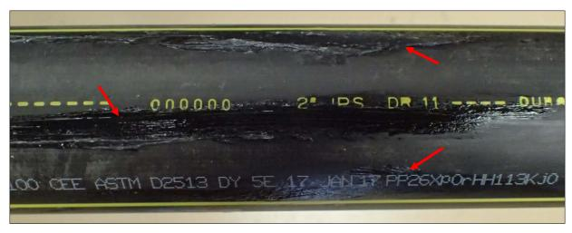
Figure 18. Test Matrix 6 specimen after silicone grease contamination, red arrows point to the three lines
