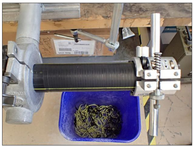
Figure 165. Pipe contaminated with bentonite powder, end of scraping pass
