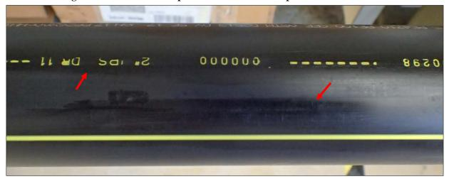
Figure 20. Test Matrix 6 specimen after water wash and wipe. Red arrows show remaining silicone grease streaks.
