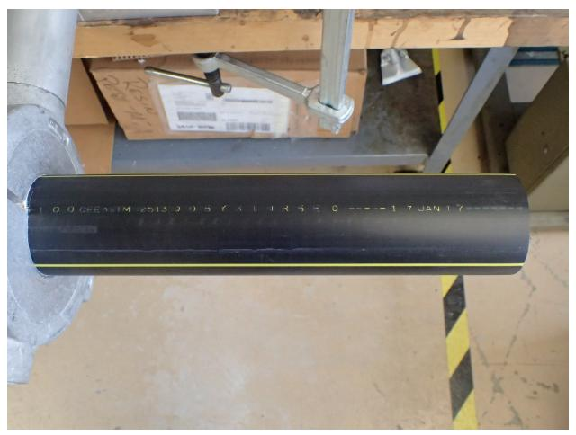
Figure 164. Pipe contaminated with bentonite powder, after three solvent cleaning passes, as necessary to make the surface visually appear to be clean; loose contamination has been removed
