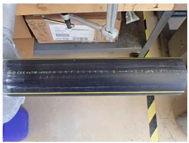
Figure 163. Pipe contaminated with bentonite powder, after two solvent cleaning passes
